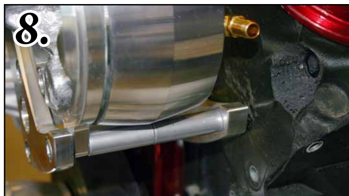
Fig. 9. Install the Alternator (P555) or (P9655) using a \frac{3}{8} x 5 \frac{1}{4} " SHCS (S279) and a \frac{3}{8} " lock nut (S622). Place a Billet Spacer Bushing (TP3-1.400) between the Alternator and the Adjust Set Screw (S450). Adjust S450 to take up any space between the lower alternator support and the spacer. (snug only at this time). Tighten lightly at this time.
