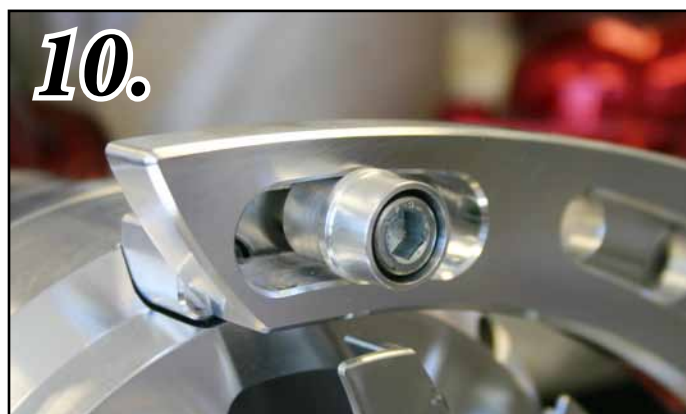
Fig. 9. Install the Alternator (P555) or (P9655) using a \frac{3}{8} x 5 \frac{1}{4} " SHCS (S279) and a \frac{3}{8} " lock nut (S622). Place a Billet Spacer Bushing (TP3-1.400) between the Alternator and the Adjust Set Screw (S450). Adjust S450 to take up any space between the lower alternator support and the spacer. (snug only at this time). Tighten lightly at this time.
