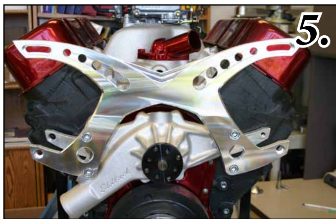
Fig. 6. Install the Adjustment Bushing (S450) into the rear Alt Support.
