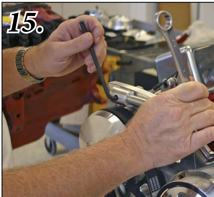
Photo 15. Use the holes in the adjustment tool to tighten both M8 socket head cap screws when correct belt tension has been achieved. Remove the adjustment tool and keep for future use.
