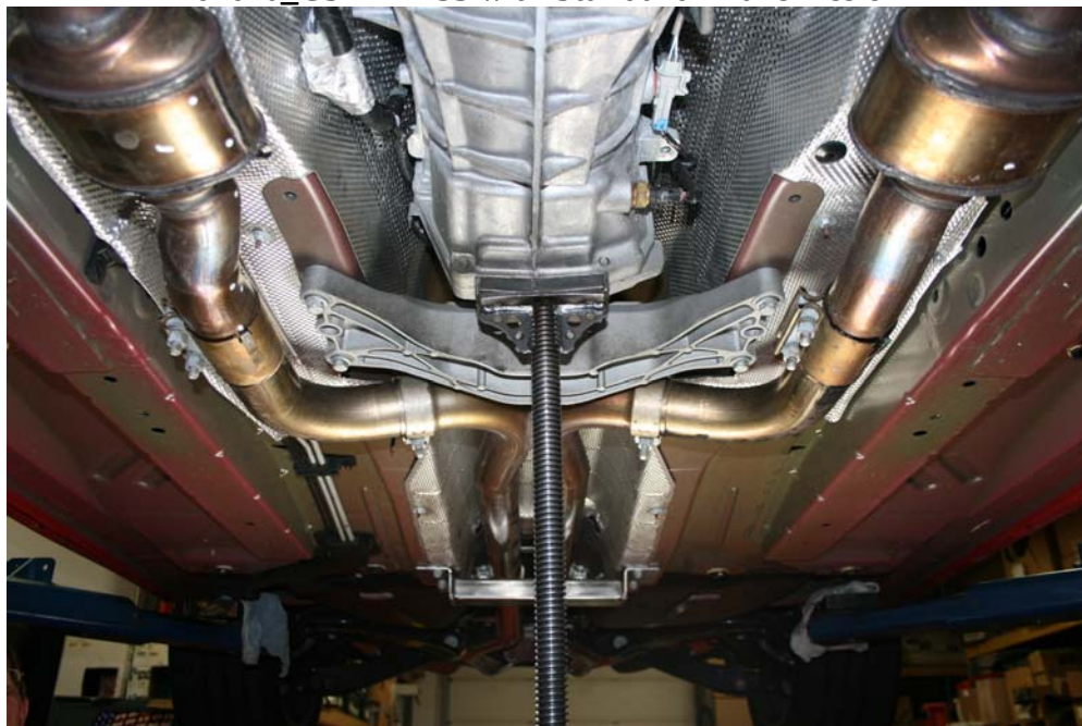
Step 1: Rear of transmission must be supported using a suitable jack
