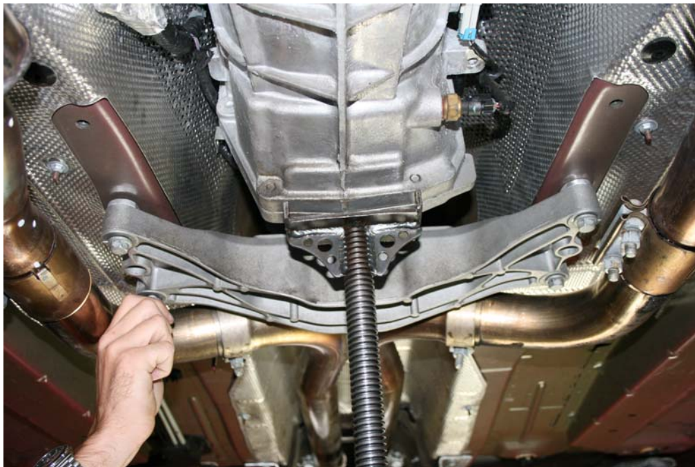
Step 8: Reinstall remaining crossmember bolts
