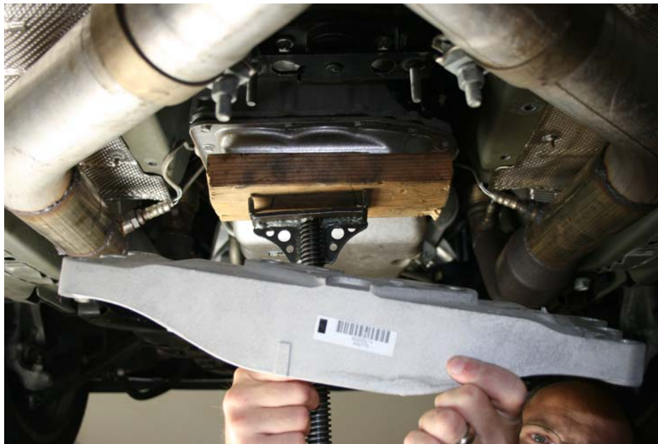
Step 4: Remove transmission crossmember from vehicle
