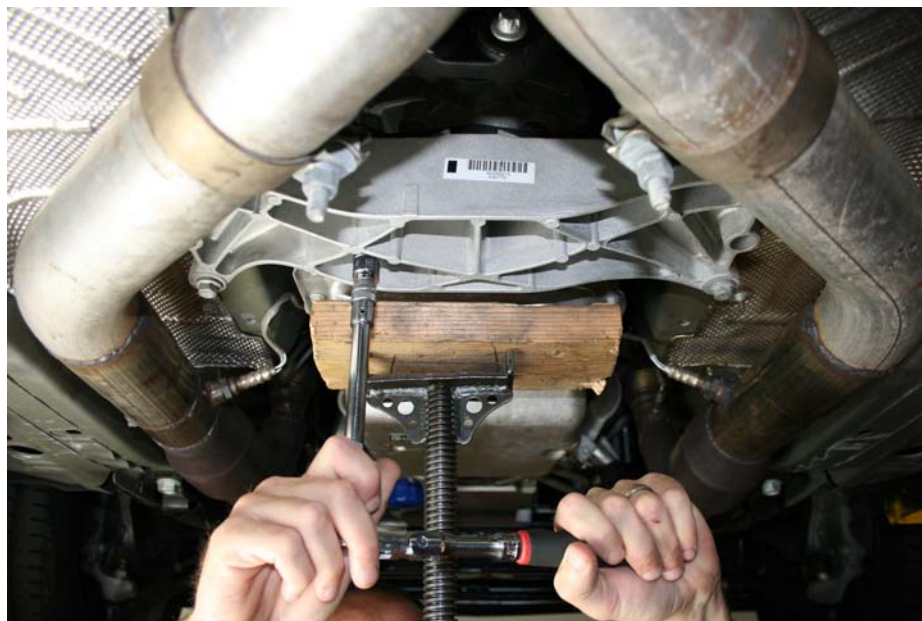
Step 2: Remove transmission mount bolts
