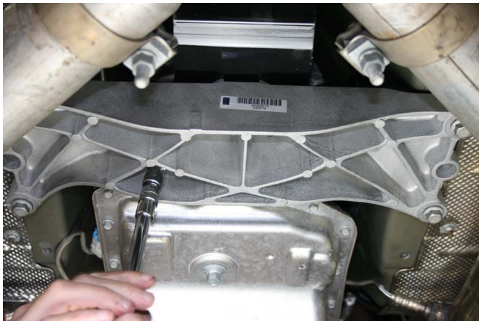
Step 9: Reinstall and tighten transmission mount bolts
