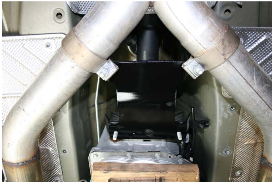
Step 6: Place drive shaft base plate over transmission mount bolts
