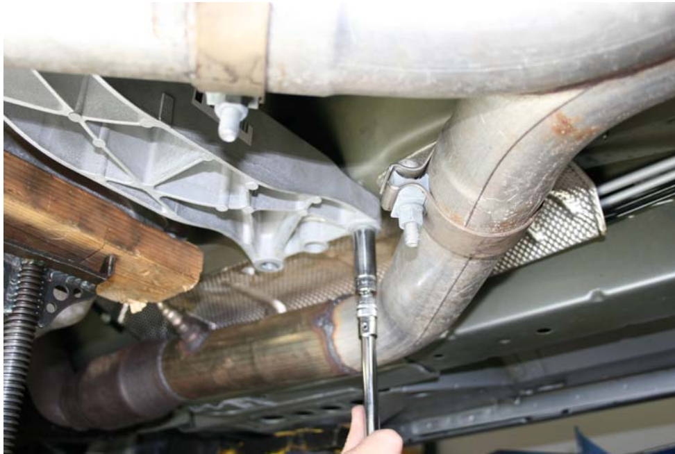
Step 3: Remove transmission crossmember bolts
