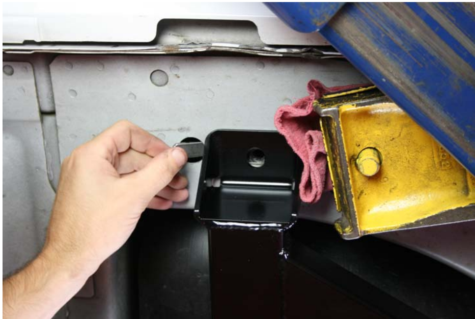
Step 6: Install ½-20 nut plate.
