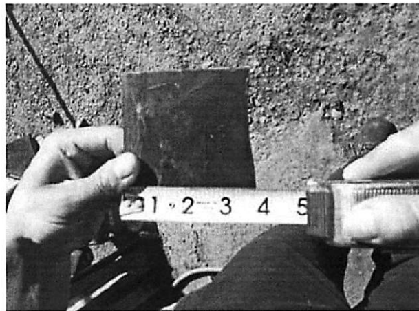
Step 23: Using some of the excess material from the blower motor housing modifications, cut a rectangle section approximately 4 x 3 1/2 inches. This will be used inside the new cover to help seal the modified blower motor housing and enhance airflow.
