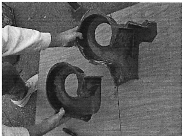
Step 18: This is a backside view of the modified housing compared to the original on the right.
