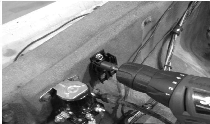
Figure 7-6 Installing the Maxi Fuse Holder '73-'77 Model
