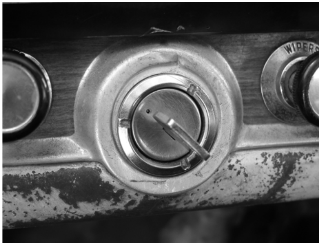
Step 1 – Turn Switch to ACC. POSITION
