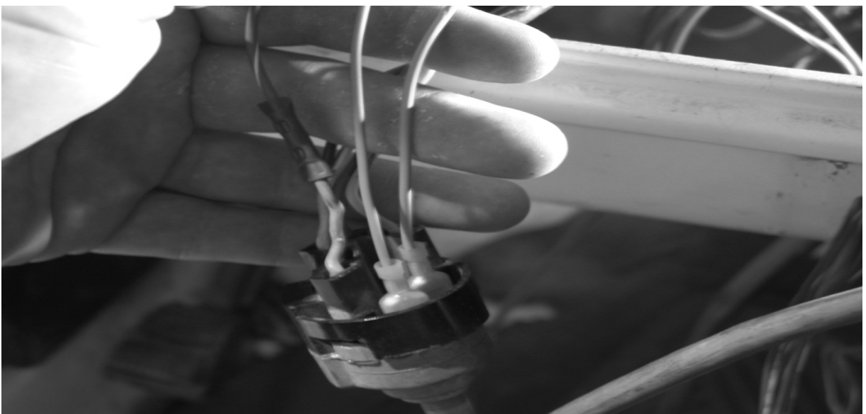
Figure 7-21 Wiper Switch w/wires connected
