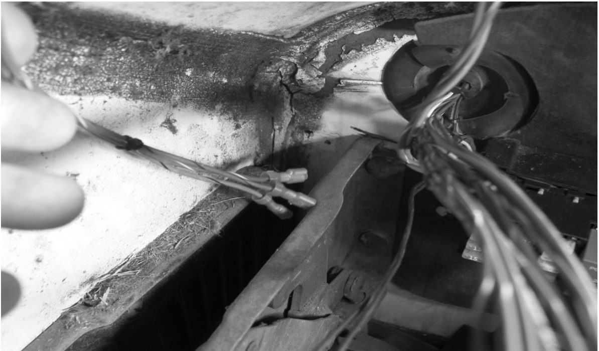
Figure 7-22 Routing the Dimmer Switch Wires
