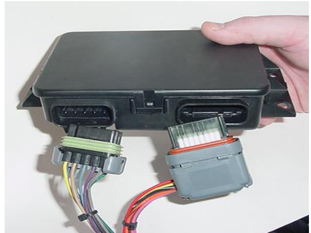
FIGURE 6.22 TAC Module Connections
