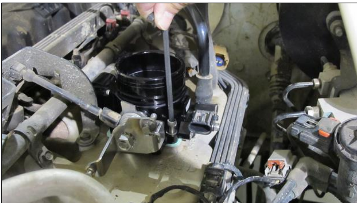
(Figure 3-19) Use a cross pattern to torque the new 8mm X 30mm mounting screws and washers to 10in/lbs.
