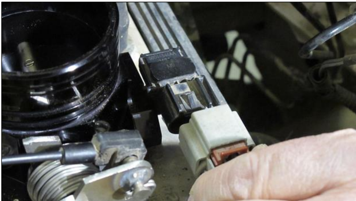
(Figure 23) Reconnect the MAP Sensor connector as shown above .
