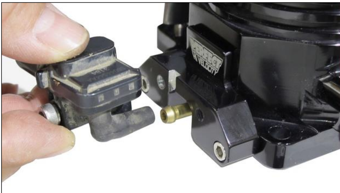
(Figure 3-16) Install the (MAP) Sensor on the new Throttle Body lining up the groove with the MAP sensor protrusion using the new #10-32 X 1-1/4" fastener provided.
