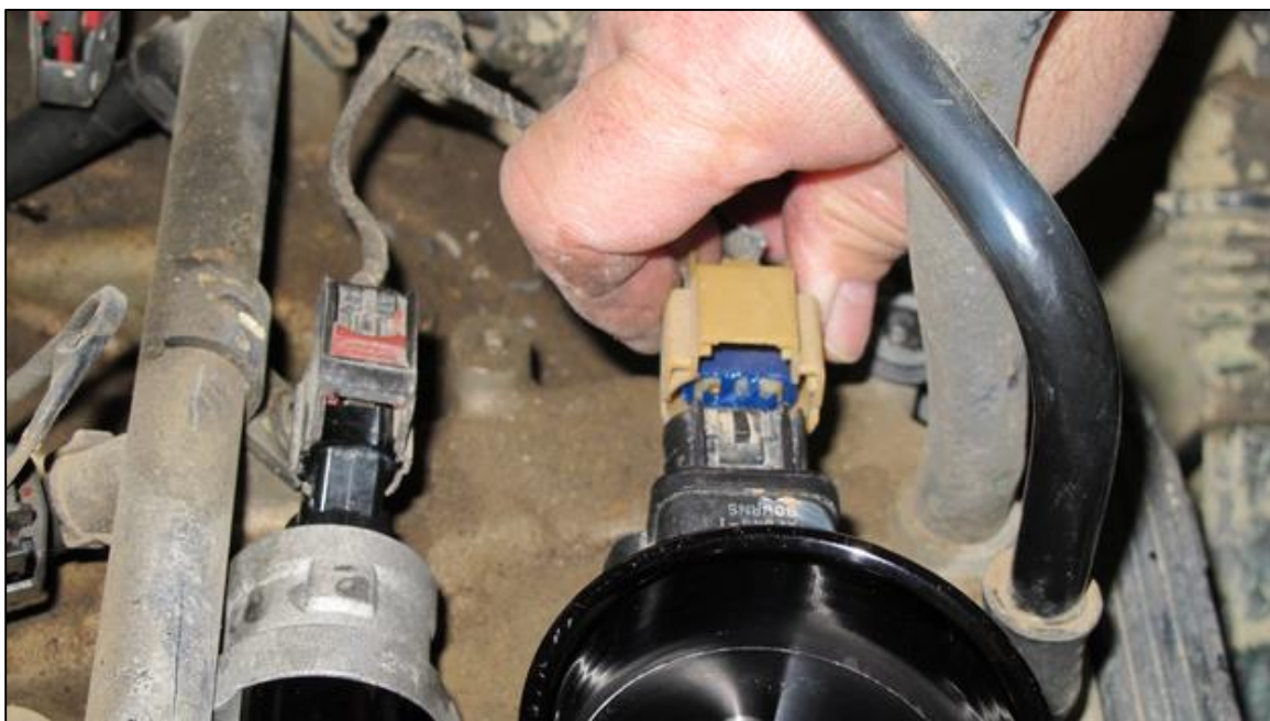
(Figure 3-20) Reconnect the TPS connector as shown above.
