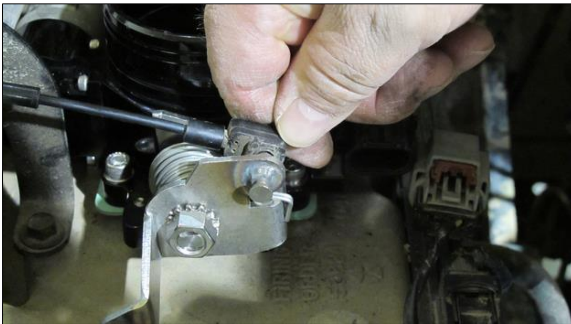
(Figure 3-18) Attach Throttle Cable to the new Throttle Body
