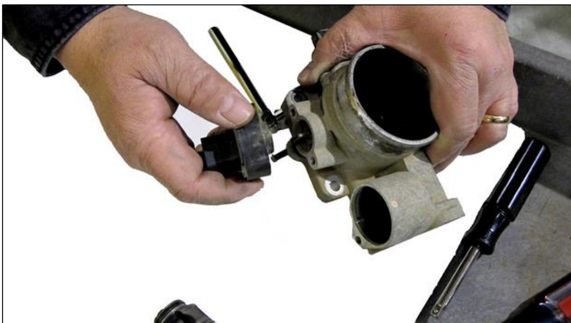
(Figure 3-9) Remove the Throttle Position Sensor (TPS) from the Throttle Body using a T20 Torx wrench or socket.
