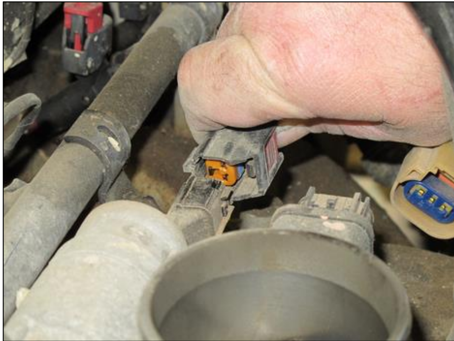
(Figure 3-5) Disconnect the electrical connector attached to the Idle Air Control Motor as shown above.
