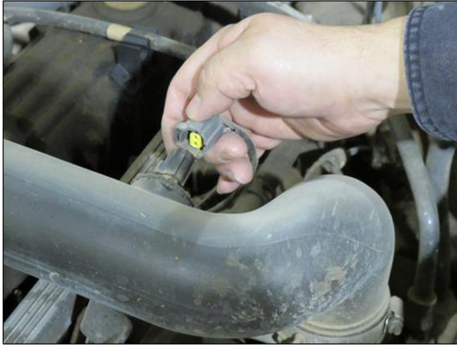
(Figure 3-1) Disconnect Intake Air Temperature Sensor (IAT).
