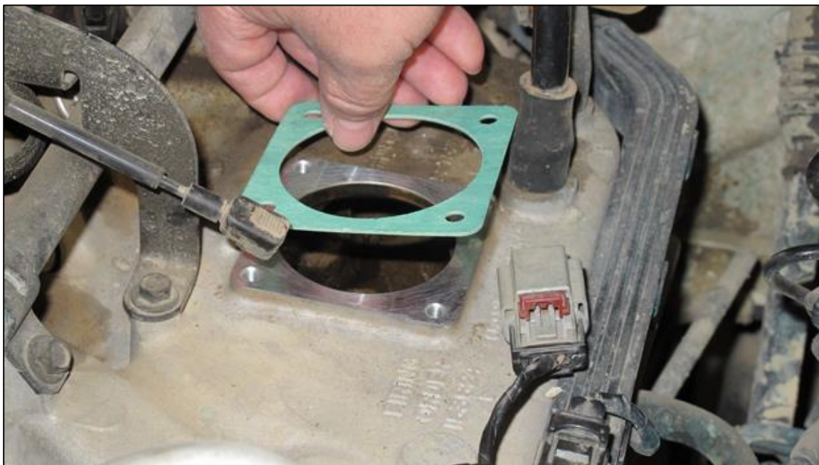
(Figure 3-17) After cleaning the gasket surface place the new throttle body gasket on intake to make ready for the new throttle body.
