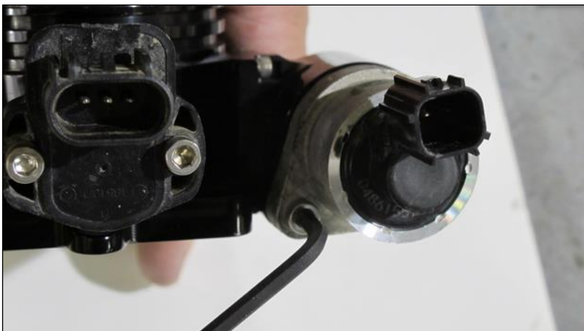
(Figure 3-15) Install the Idle Air Control (IAC) motor on the new Throttle Body, using the new #10-32 X 1/2" fastener provided.
