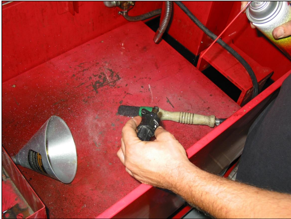
(Figure 3-13) Clean the IAC motor by spraying carburetor cleaner on it carefully wiping it clean.
