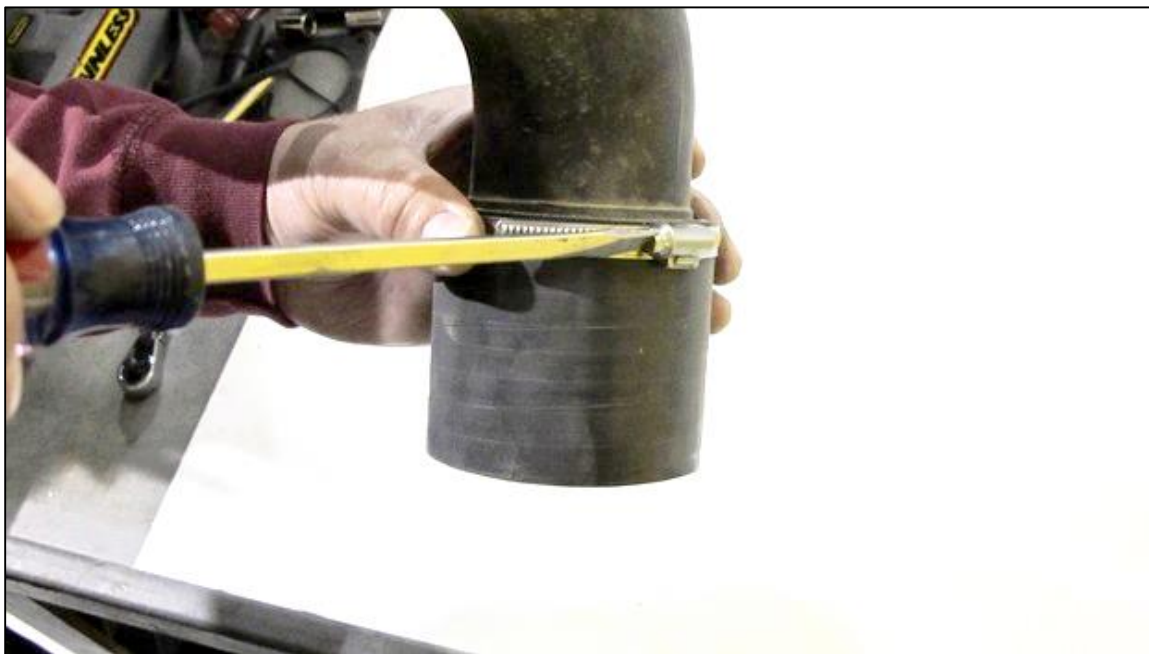
(Figure 3-25) You will clamp the adapter onto the hard plastic section of the factory air intake tube for a good seal as shown above. Do not over tighten and damage the tube.
