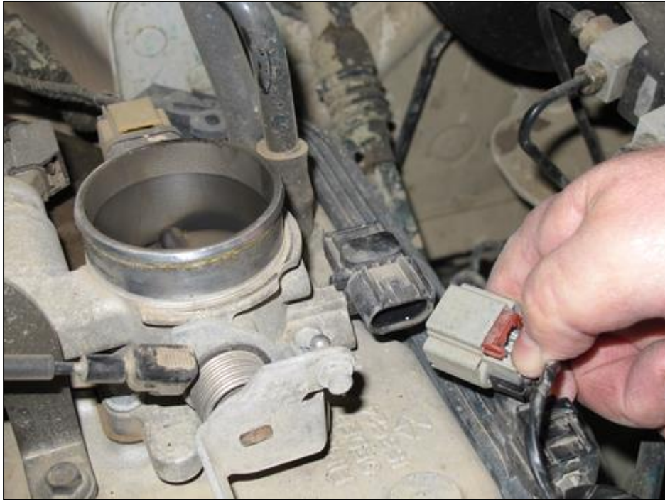
(Figure 3-7) Disconnecting the Manifold Absolute Pressure MAP sensor
