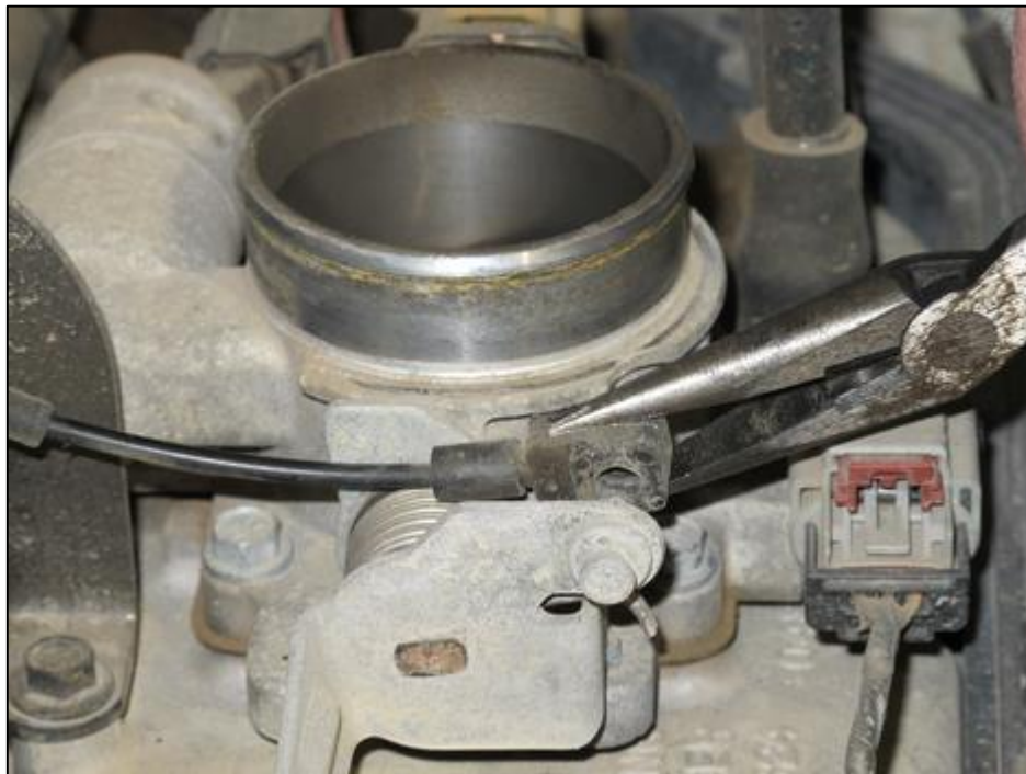
(Figure 3-4) Carefully pry off the ball-type throttle cable linkage with a pair of needle nose pliers.
