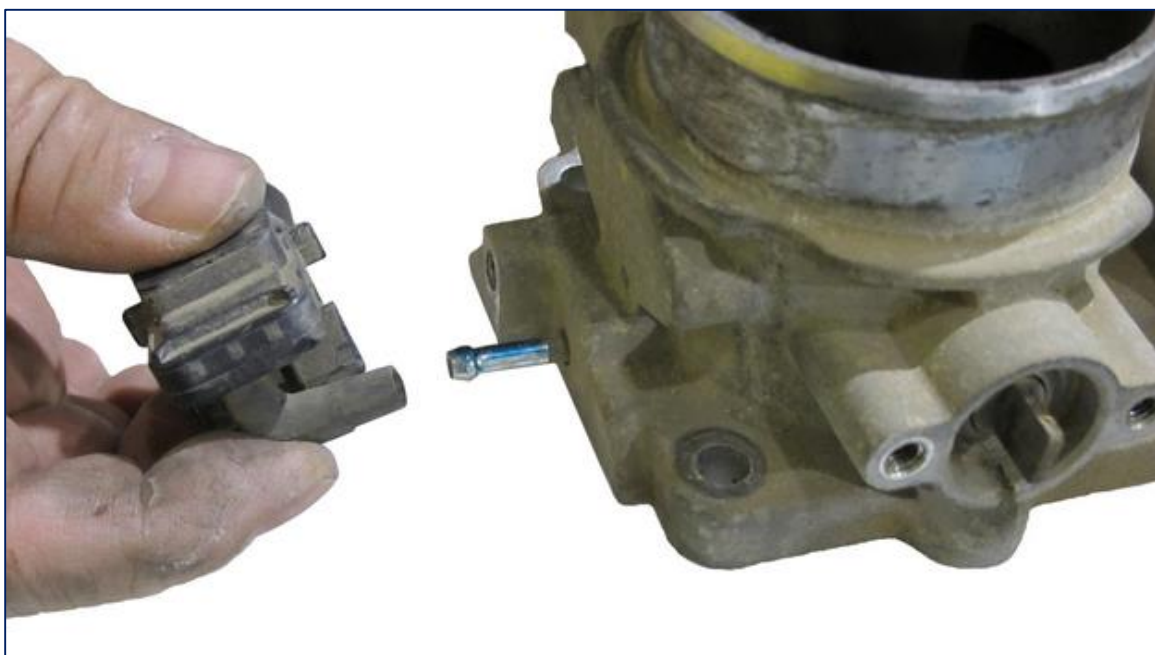
(Figure 3-11) Remove MAP Sensor inspect vacuum tube for damage replace if necessary.
