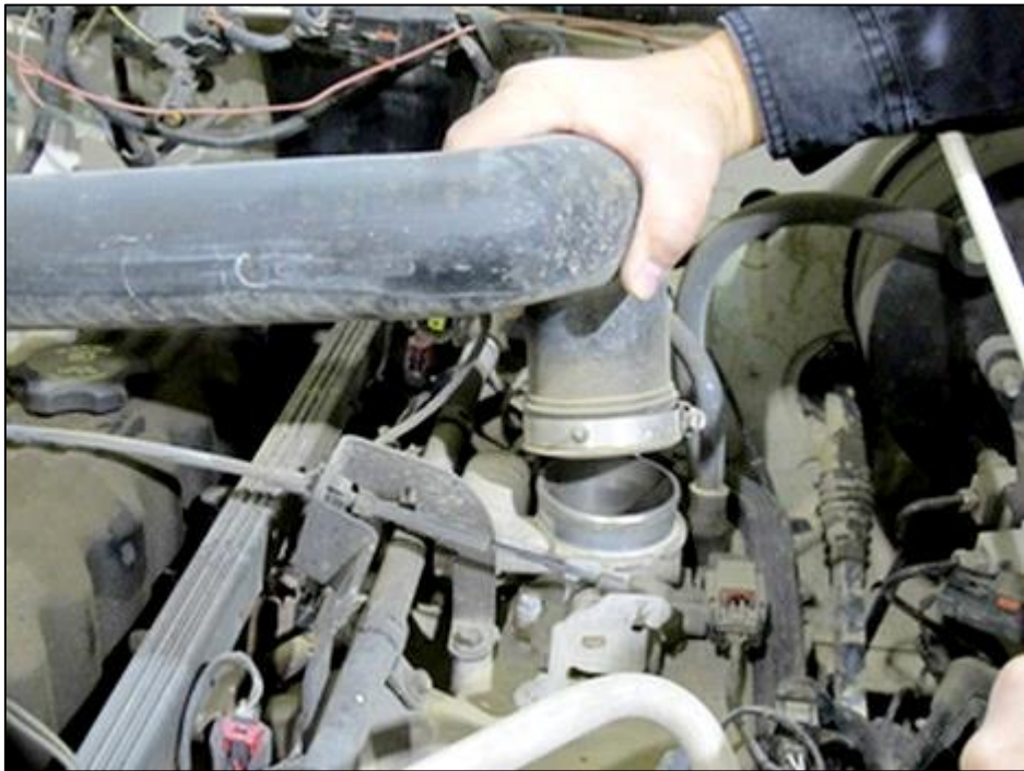
(Figure3-2) Remove factory air intake tube from throttle body.
