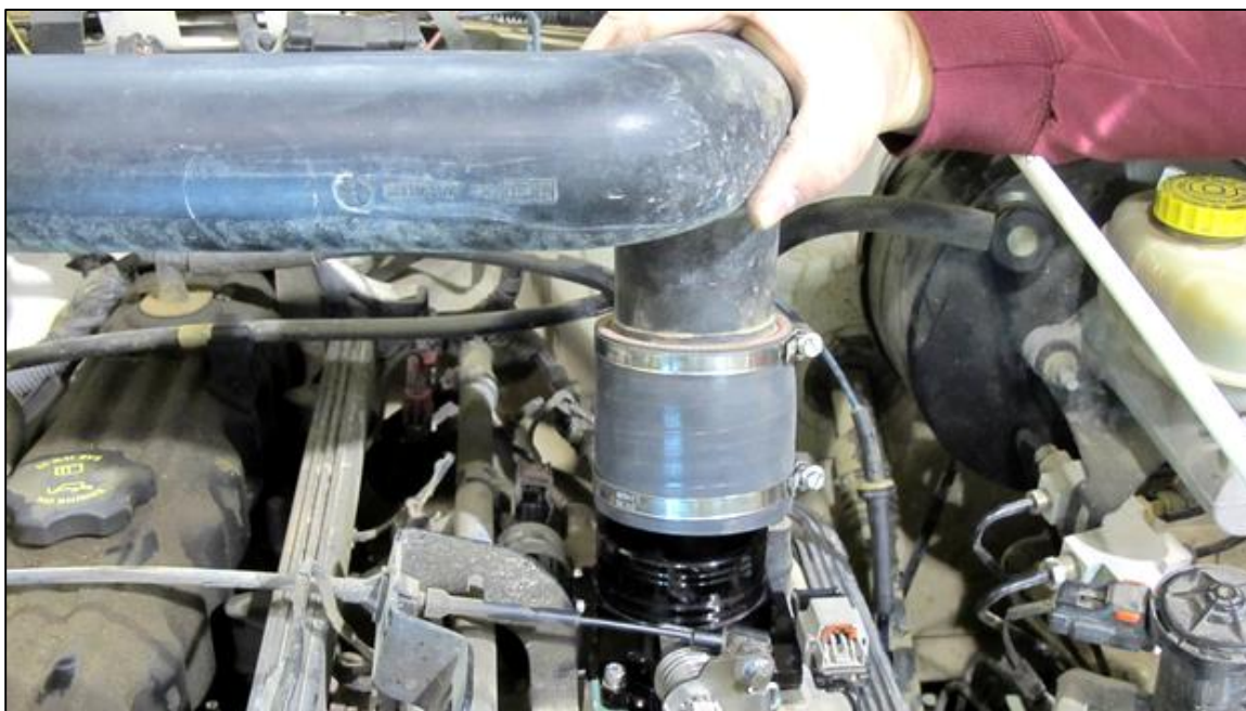
(Figure 3-26) Refit the air intake tube as shown above and secure clamp to Throttle Body.
