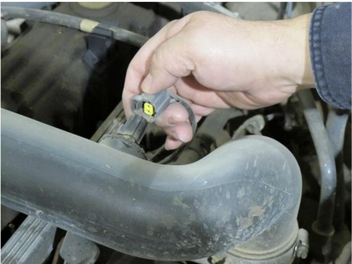
(Figure 3-28) Reconnect the Intake Air Temperature Sensor (IAT) as shown above.
