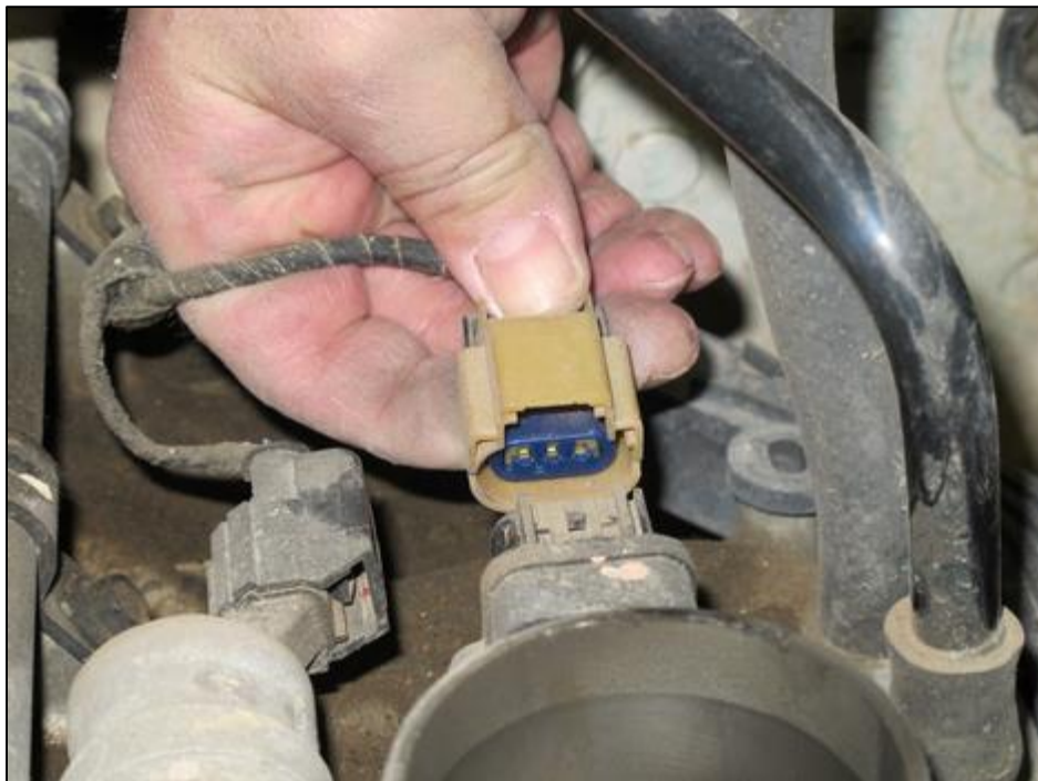
(Figure 3-6) Disconnecting the Throttle Position Sensor (TPS)
