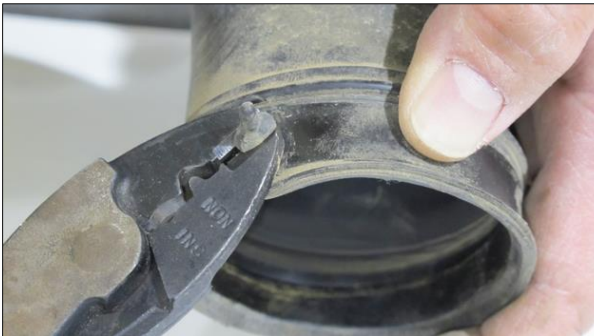
(Figure 3-22) Re-install the air intake tube using the adapter provided. You will clamp the upper part of the adapter to the hard plastic section of the factory tube for a good seal. You must trim the factory clamp position locator as shown above.
