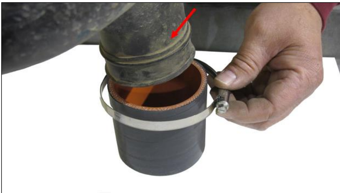
(Figure 3-24) Secure the new clamp above the 2 ridges on the hard plastic portion of the factory air tube as shown in figure 3-25.
