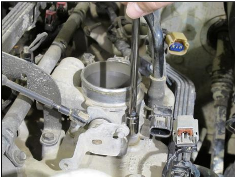
(Figure 3-8) Using a 10mm socket on a 6" extension, remove the (4) Throttle Body bolts and remove the throttle body from intake manifold.
