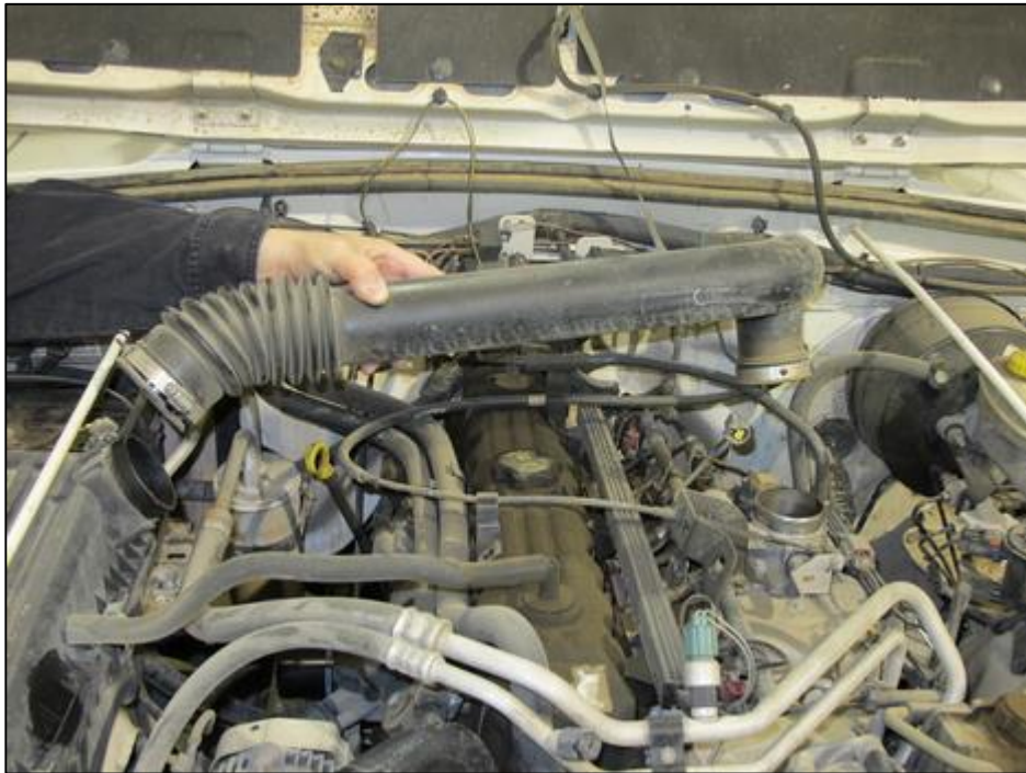
(Figure 3-3) Air Filter and Intake Tube Removal
