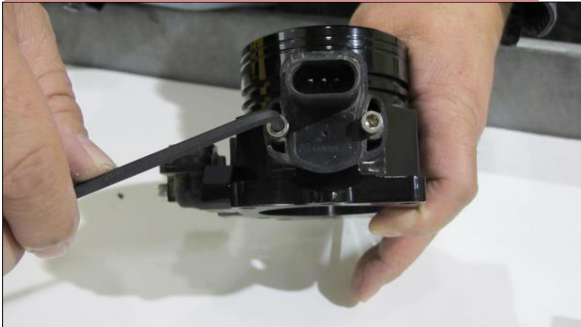
(Figure 3-14) Install the new TPS onto the new throttle body using the new #10-32 X 3/4 fasteners provided.
