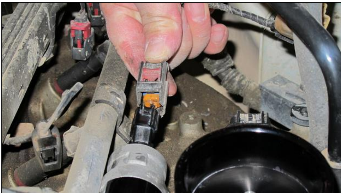
(Figure 3-21) Reconnect the IAC connector as shown above.
