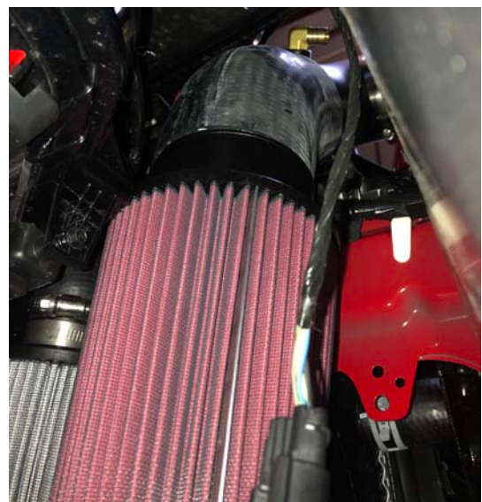
Air Filter Installed
