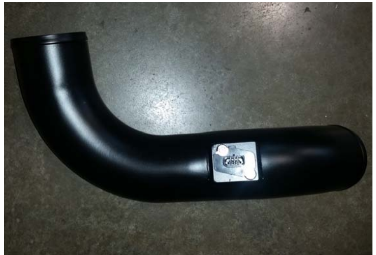
MAF Installed Into Tube #430
