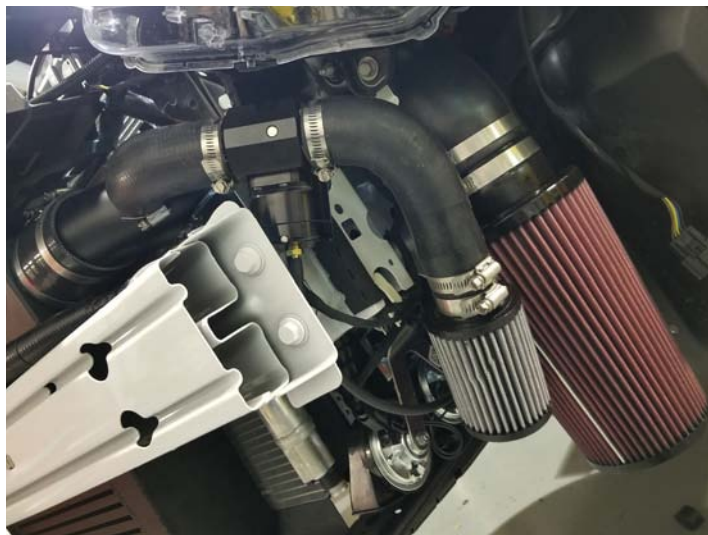
ProFlow Surge Valve Installed
