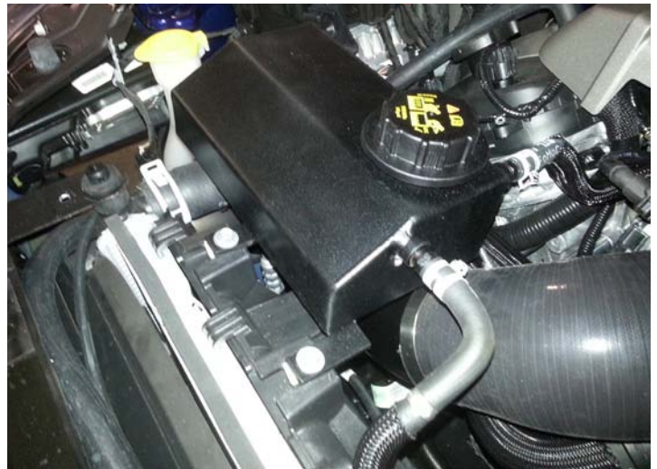
New Coolant Reservoir Mounted
