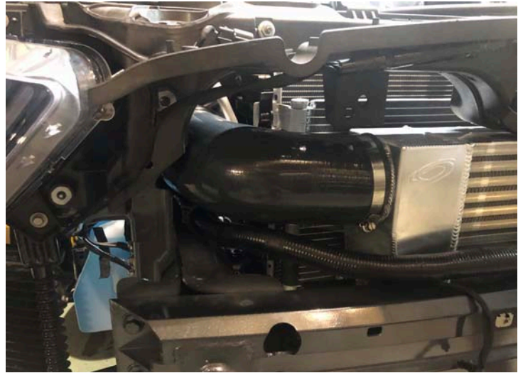
3.5" 90° Silicone Elbow Installed
