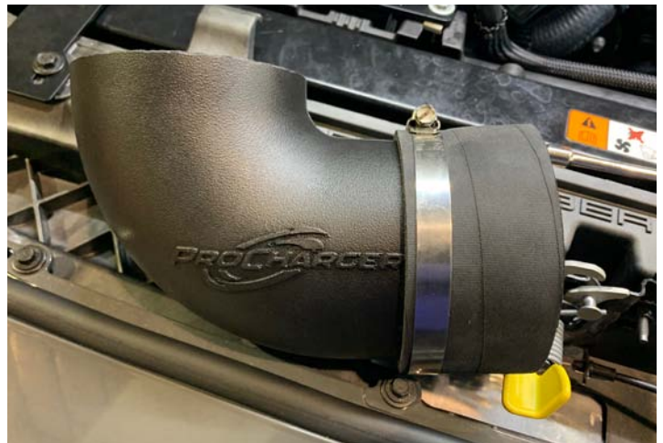
Plastic Inlet Installed
