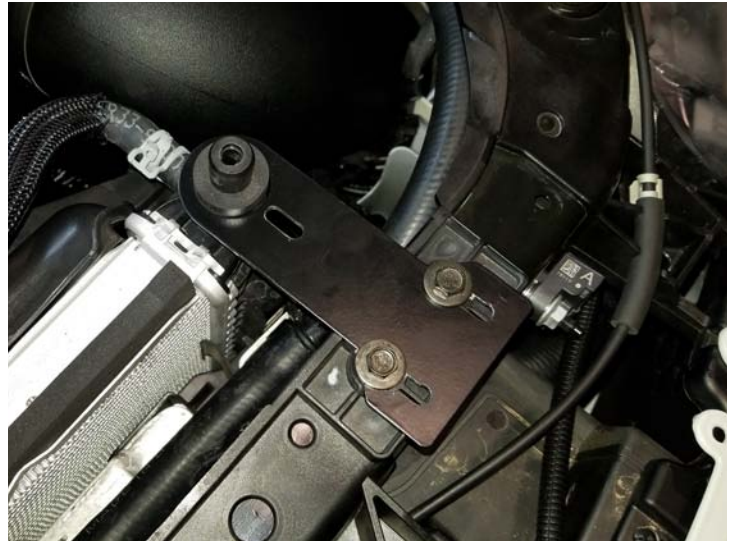
Radiator Bracket Installed
