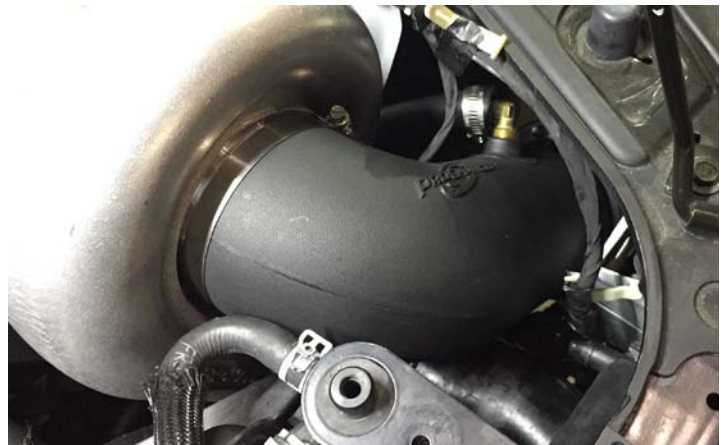
Inlet Elbow Installed
