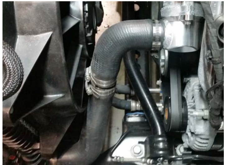
Upper Hose Section Installed
