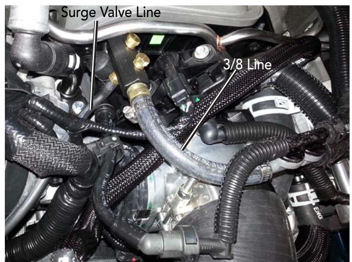
Vacuum Manifold Installed
