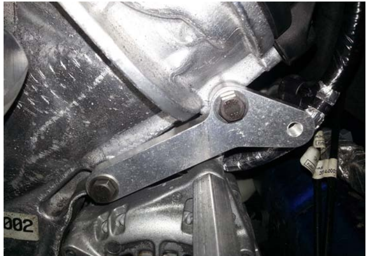
Sub Bracket Installed
