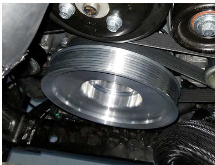
Crank Pulley Installed
