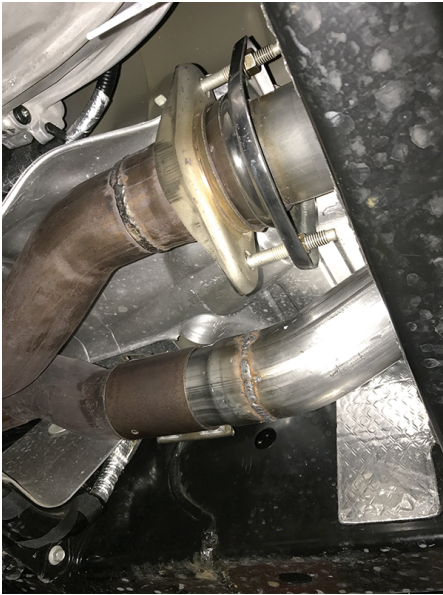
Image A: Front clamp location and orientation
