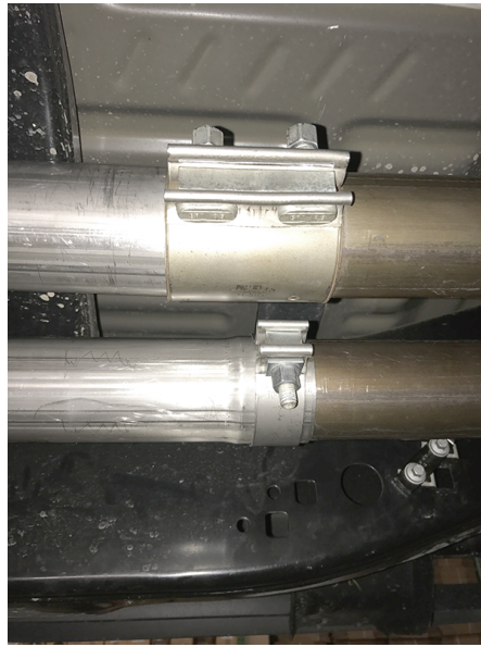
Image B Rear clamp location and orientation
