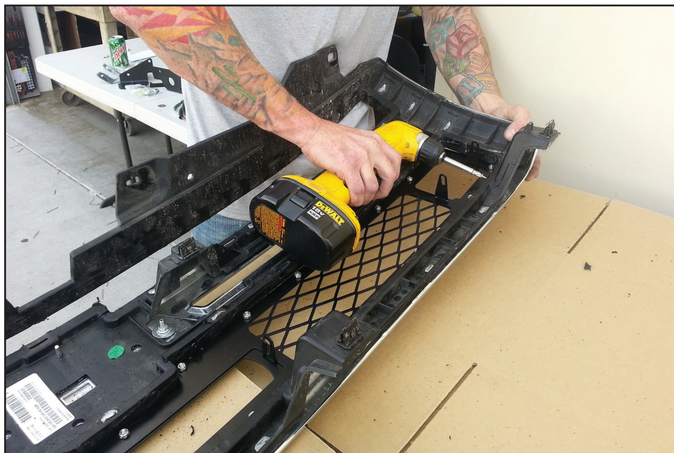
Attach grille to grille shell using nuts & bolts OR self tapping screws.
