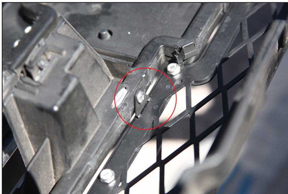
Self tapping screw shown attaching grille insert to grille shell using mounting tabs.
