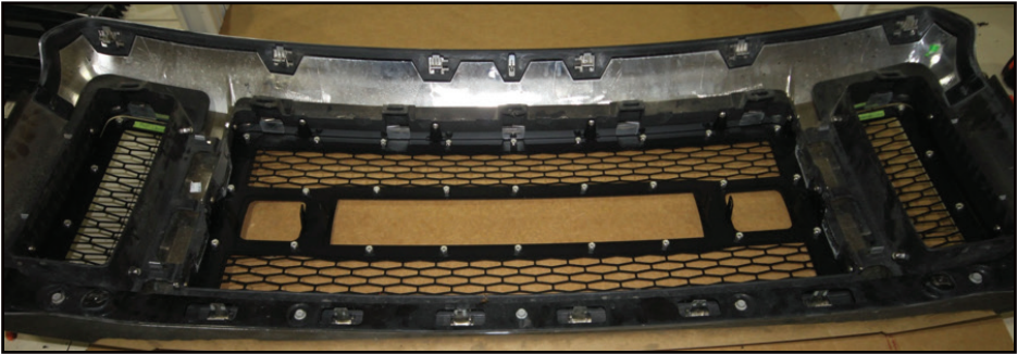
Secure Grille Pieces to Shell with 1/4" Bolts/Nuts
