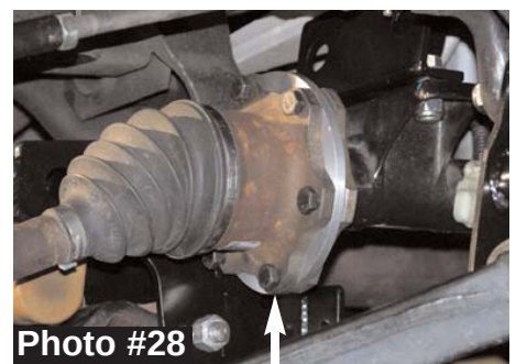
Passenger side shown with one 15/16" C.V. spacers.
