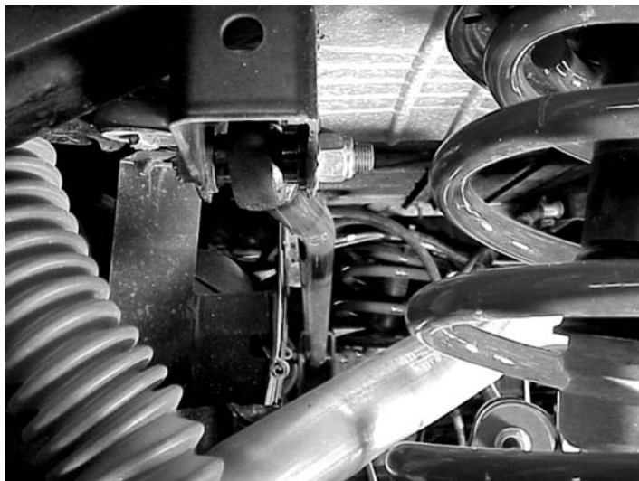
Rear Trackbar installed (notice the location of the bend)
