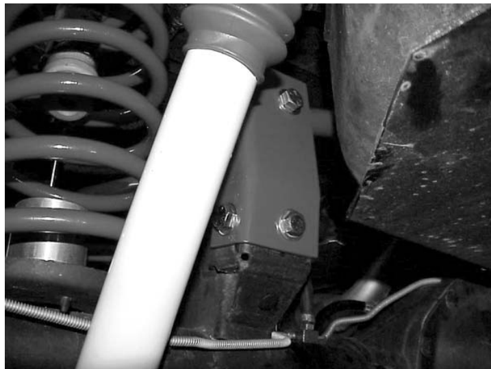
Rear Trackbar Bracket (installed) driver side view
