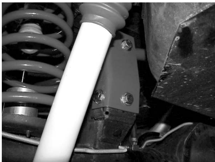
Rear Trackbar Bracket (installed) driver side view
