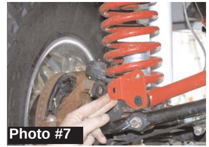
5/16" x 3/4" thread cutter flange bolt.
