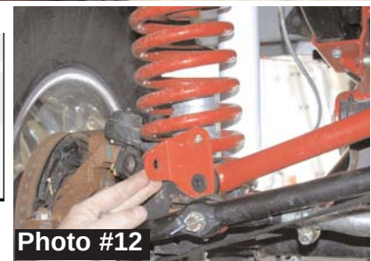
5/16" x 3/4" thread cutter flange bolt.
