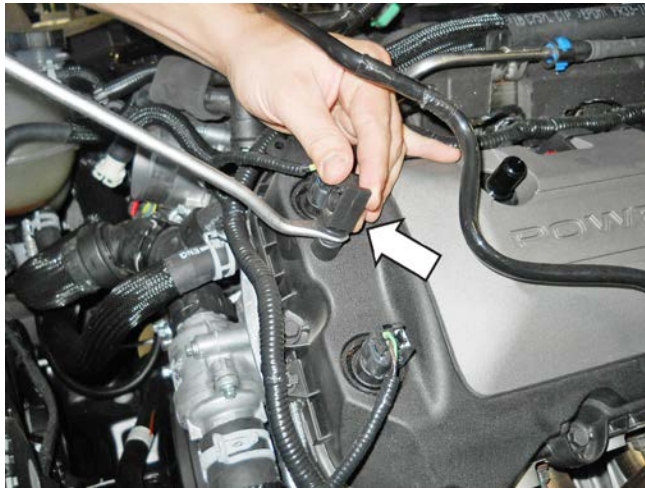
Remove retainer on cam cover
