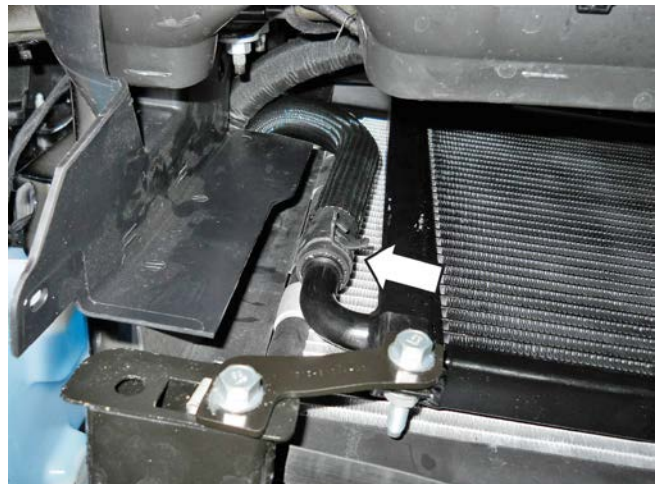
Pump hose to LTR connection
