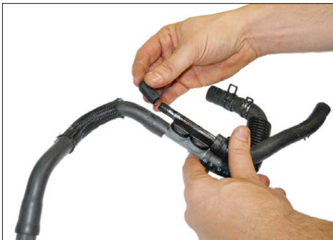
13. On hose 4, remove the convolute off of the curved end.
