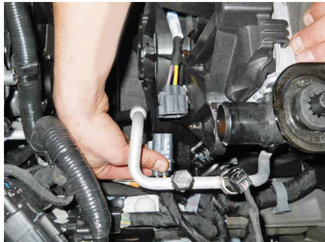
Fan shroud electrical connector
