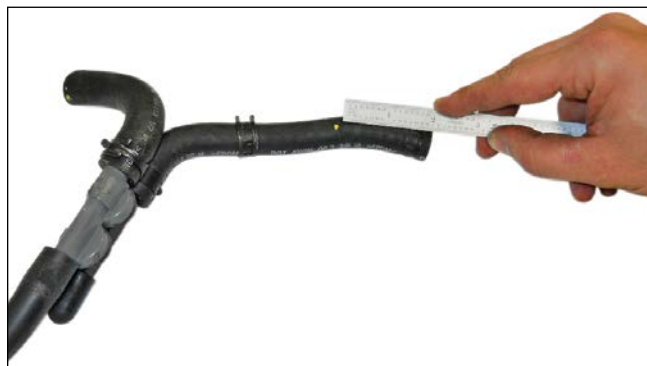
17. On hose 2, mark and cut 2" from the end of the hose.
