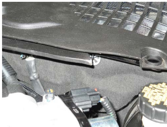
Exposed point on modified K-brace, shown installed
