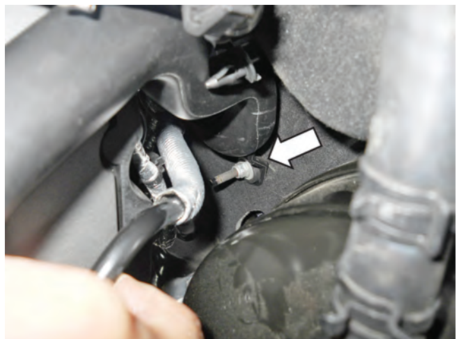
Showing nut at firewall
