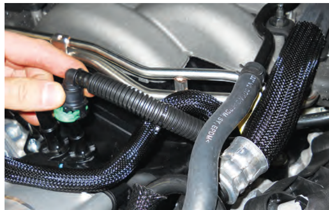
EECPV tube quick connector with green lock
