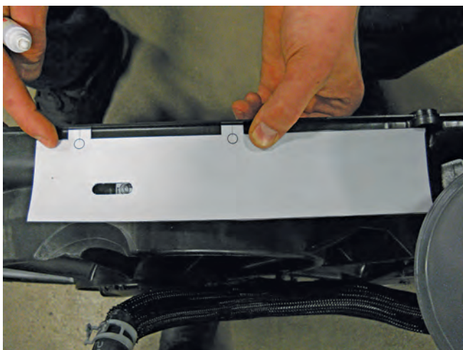
Proper template position on fan shroud
