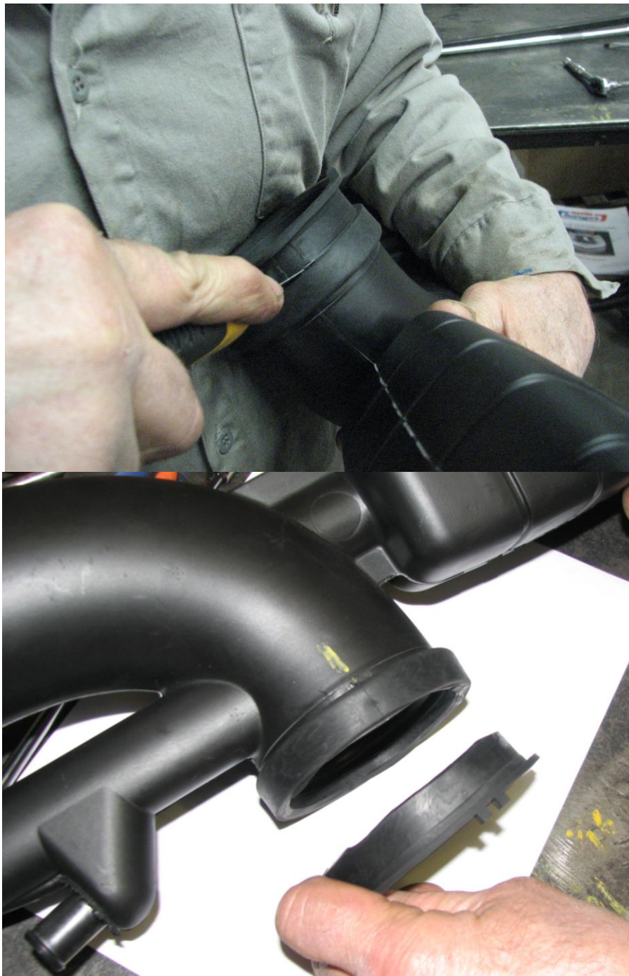
Figure 2a & 2b: Cutting of the factory air tube
