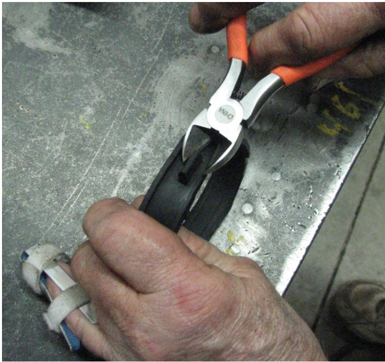
Figure 3: Cutting of the tab on 'spacer'
