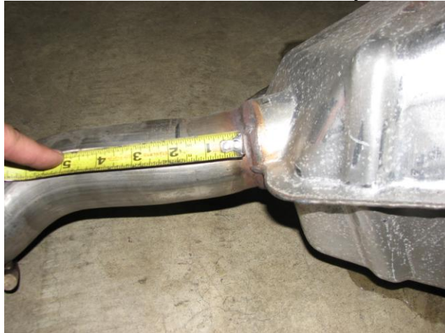
Figure 1: 1.75" from weld on rear muffler
