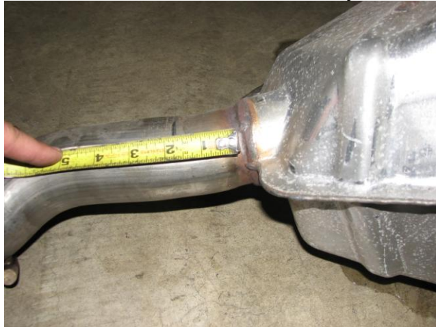
Figure 1: 1.75” from weld on rear muffler
