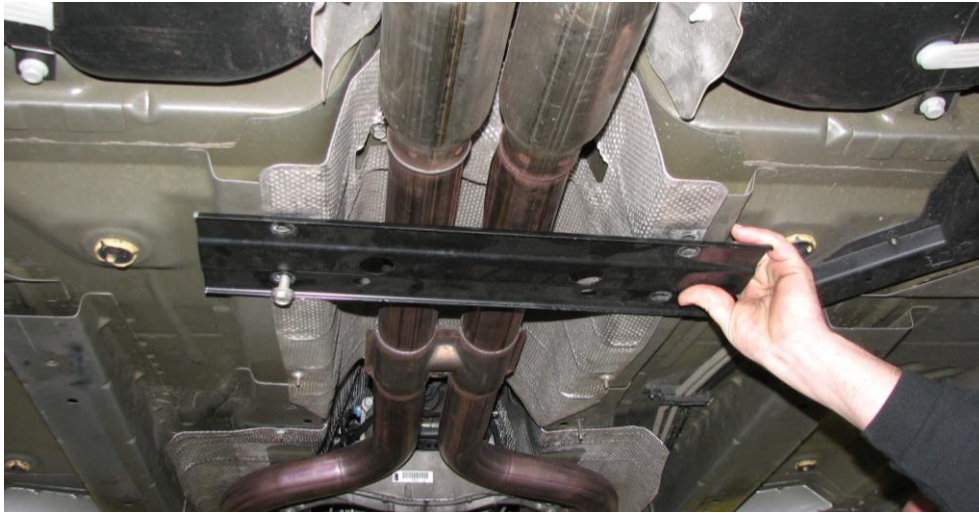
Figure 1: Removal of tunnel brace
