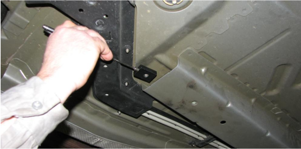
Figure 3: Feeding thread plate down frame rail using magnet
