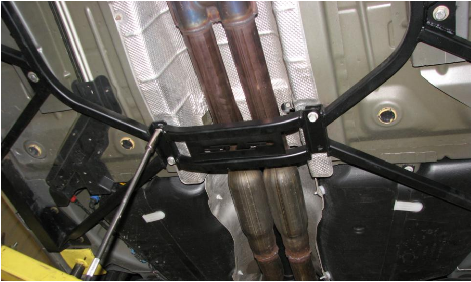
Figure 7: Installation of SLP tunnel brace
