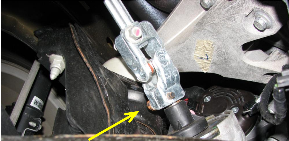
Figure 1: Remove this bolt from steering shaft
