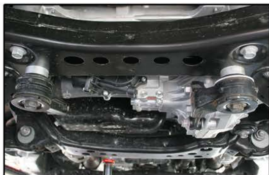
Fig. 10: All Spacers Installed
