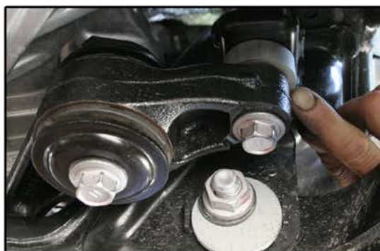
Fig. 9: Torque Arm Bracket & Spacer Installation
