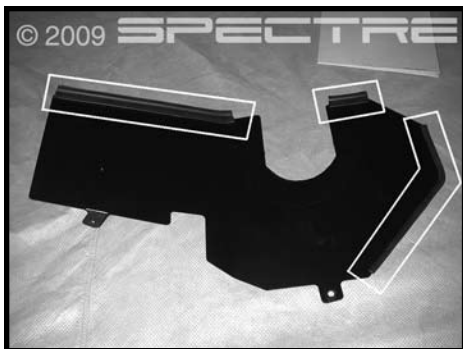
Step 7 Install the small rubber liner and rubber seals on the heat shield.
