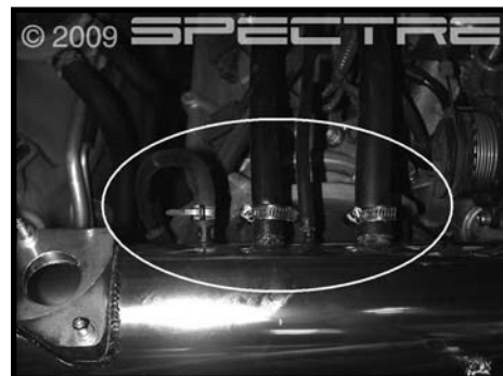
Step 14 Install the 3 new hoses and the factory hose (removed in step 5) and secure in place using the supplied hose clamps. If the vacuum cap was removed in step 4 install that now (there will be 3 hoses and 1 vacuum cap).
