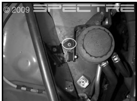
Step 8 Remove the nut on the power steering reservoir bracket. Remove the bolt on the bracket (shown above). Insert the heat shield and use the stock nut and bolt to secure in place.
