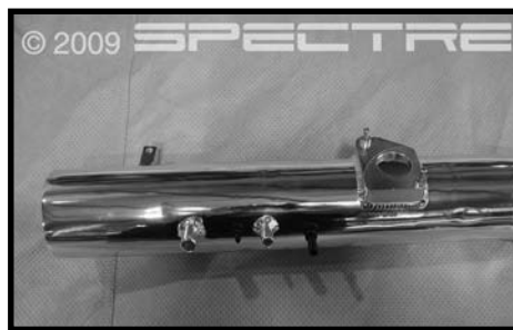
Step 10 Install the two supplied grommets and hose nipples onto the intake tube.
