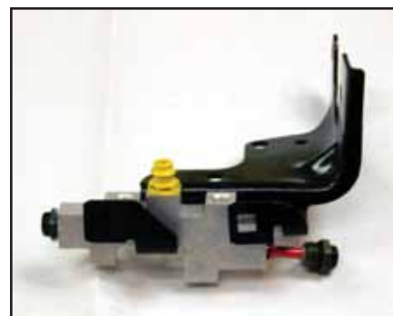
Replace endnut and piston into distribution block.
