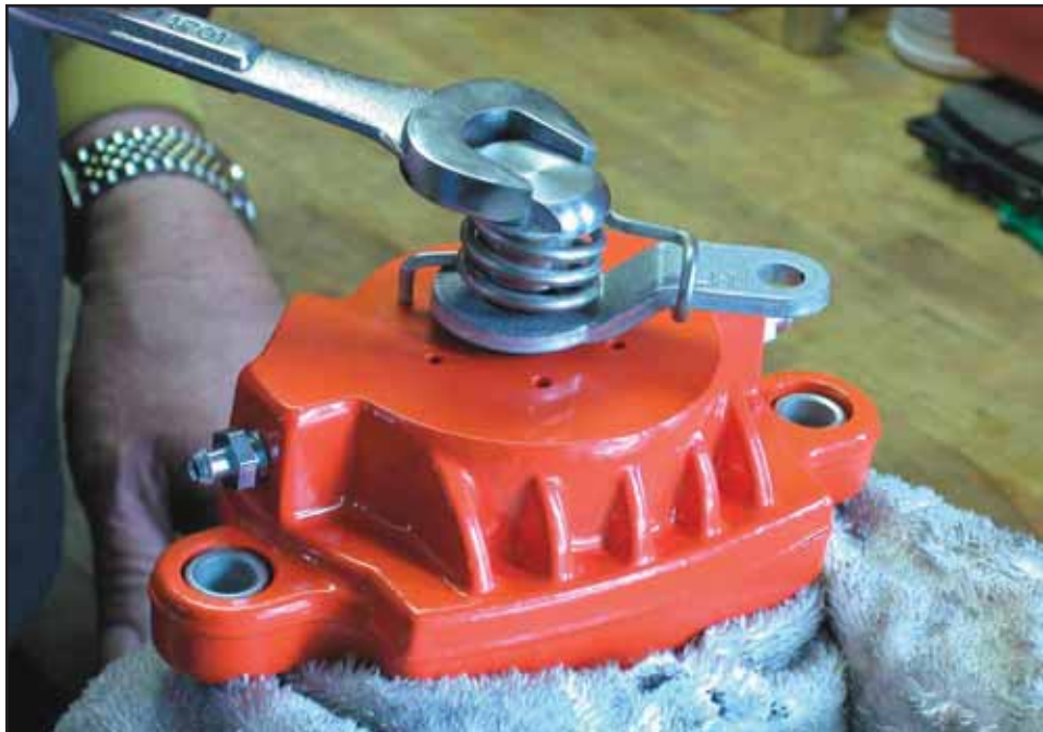
Photo 2: Using a 3/4" open end wrench, loosen and remove the retaining nut.
