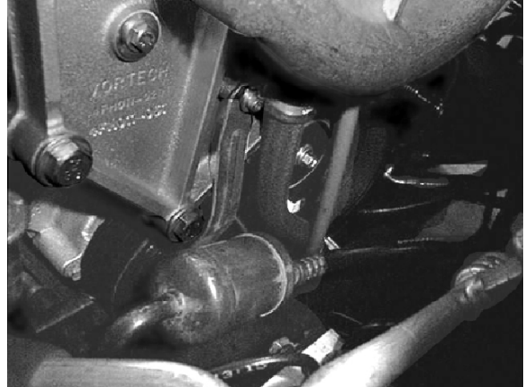
Fig. 8.2-g / Air Conditioning Silencer
