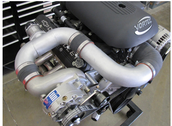
Fig. 3-d: Install Discharge Tube B
