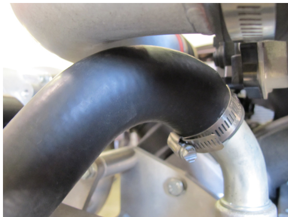
Fig. 4-d: Install Modified Coolant Hose Elbow
