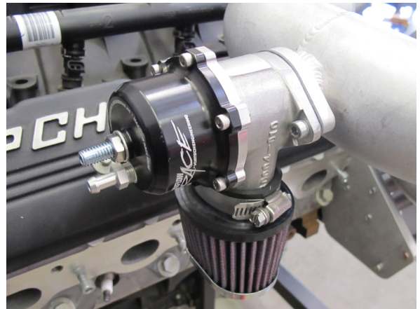
Fig. 3-e: Install Bypass Valve
