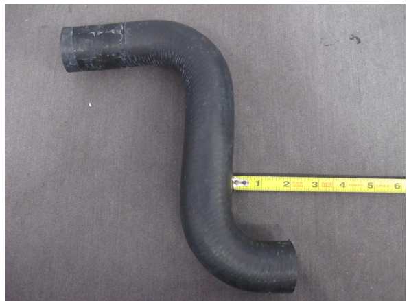
Fig. 4-c: Modified Coolant Hose
