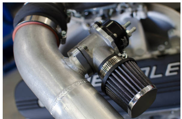
Fig. 3-i: Install Bypass Valve
