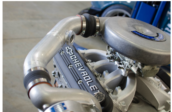
Fig. 3-h: Install Discharge Tube
