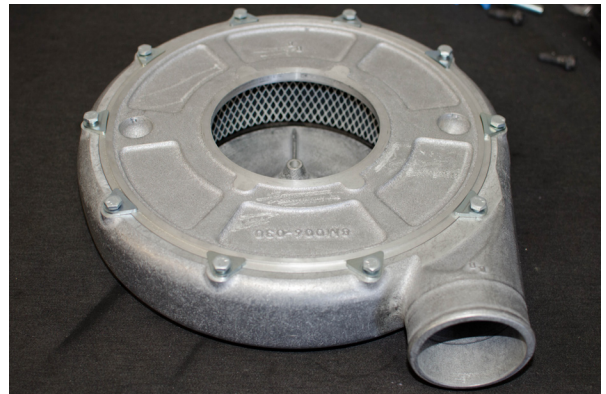
Fig. 3-b: Re-install Carburetor Hat Base
