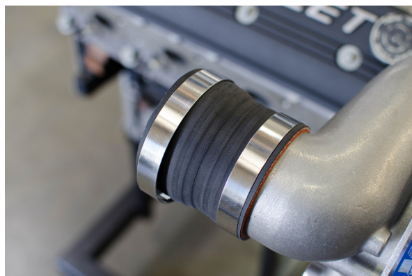
Fig. 3-f: Install 3.00"-2.75" Reducer Sleeve
