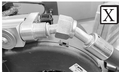
Improperly Seated O-ring Land
