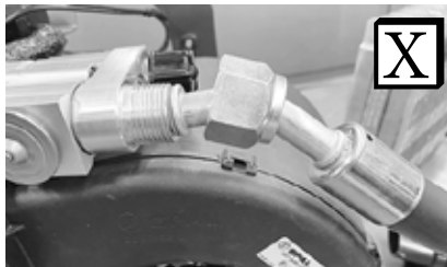
Improperly Seated O-ring Land
