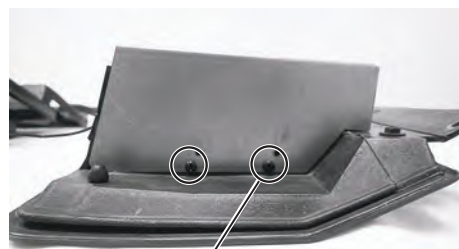
Install glove box cap using (4) #6 x 3/8" pan head screws
