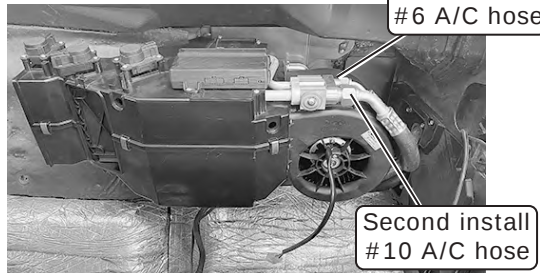
A/C Hoses Installed
