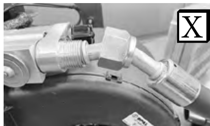
Improperly Seated O-ring Land
