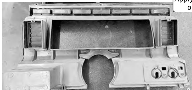
Foam Removed from Driver-Side Louvers
