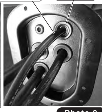
#6 Drier/Evaporator A/C Hose
