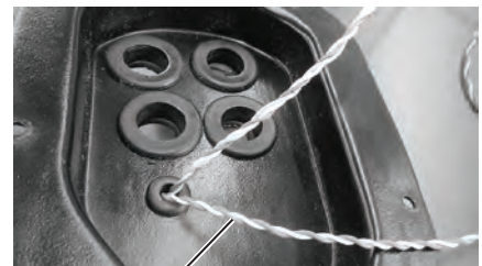
Route red, white and blue wires from main harness through 7/8" wiring grommet on kick panel cover
