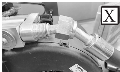
Improperly Seated O-ring Land
