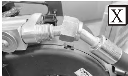
Improperly Seated O-ring Land
