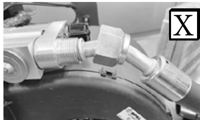
Improperly Seated O-ring Land
