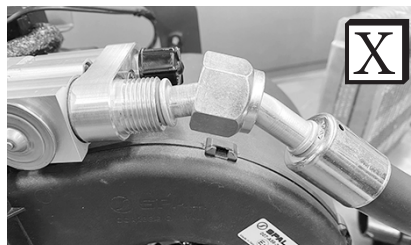
Improperly Seated O-ring Land
