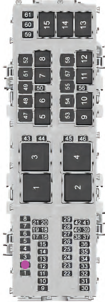
MAIN FUSE PANEL BEHIND CENTER CONSOLE
