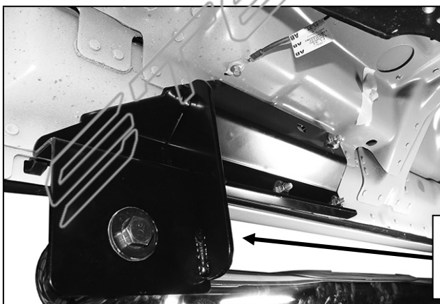
(Fig 5) Passenger side front Bracket installation
