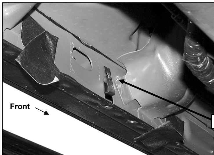
(Fig 4) Driver side-center Mounting Bracket location
