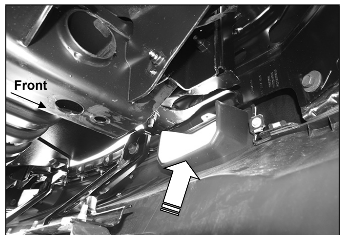
(Fig 4A) From behind bumper, insert passenger/right Frame Bracket up and out through opening (Silverado model used for instruction purposes)
