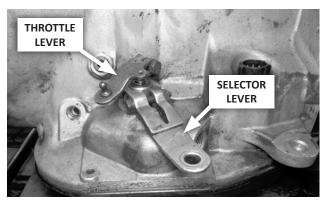
**12.** Disconnect stock controls: Loosen the throttle lever pinch bolt, remove the lever from its shaft, and carefully move the lever and linkage aside, allowing them to hang free. Remove and discard the stock selector lever and shift linkage.
