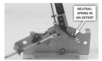
A. Manually move the selector lever to the NEUTRAL detent (2 clicks back from full-forward), and move the shifter to the NEUTRAL position. Adjust cable bracket nuts (and the swivel, if necessary) until the swivel slips freely in and out of the selector lever hole.
