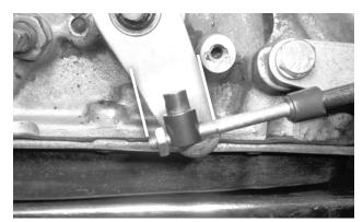
**31.** Thread the swivel onto the cable to about the middle of the threaded section, then reinstall (but do not yet tighten) the jam nut.
