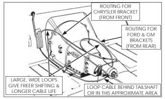
10. Route the cable approximately as shown, based on your application. Avoid any sharp bends which may kink or otherwise damage the cable. Seal the cable hole shut to keep exhaust fumes, water, etc. out of the passenger compartment. Use clamps and / or cable ties (customer supplied) to secure the cable housing in such a way as to prevent contact with the exhaust system, engine, or any moving parts.
