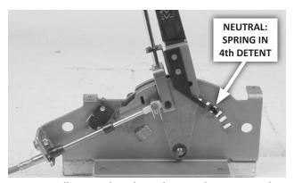
A. Manually move the selector lever to the NEUTRAL detent (3 clicks back from full-forward), and move the shifter to the NEUTRAL position (spring in 4th detent). Adjust cable bracket nuts (and the swivel, if necessary) until the swivel slips freely in and out of the selector lever hole.
