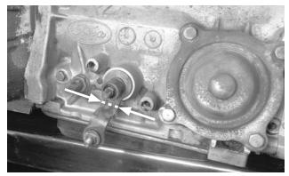
27. Move the selector lever to NEUTRAL (2 clicks from PARK). If the selector lever points downward, cut it off at the inboard bend, to allow correct positioning of the B&M lever.
