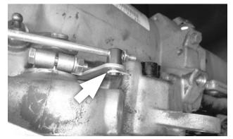
**19.** Secure the swivel to the selector lever with the **1/16**" (small diameter) cotter pin. Operate the shifter through all the gear positions, verifying that it operates correctly.
