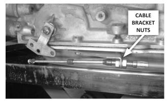
**44.** Attach the shifter cable to the cable bracket: First remove the small jam nut, both plastic dust boots, and one large nut and lock washer, from the cable. Then insert the cable through the cable bracket, reinstall the lock washer and nut (loosely, to allow room for adjustment), and reinstall the dust boots.
