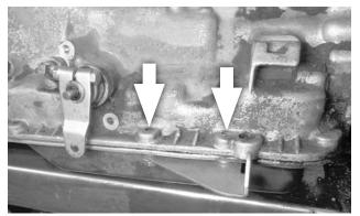
C6 transmissions: Install the cable bracket at the two left rear oil pan bolt holes, using the two 5/16-18 × 1" bolts and flat washers. For stamped sheet-metal (stock) pans, use the two spacers between the pan and bracket. (Spacers are not used with cast aluminum pans.) Tighten the bolts to 12-13 ft-lbs torque.
