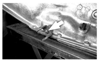
**40. Disconnect stock controls:** Remove and retain the selector lever nut. Remove and discard the selector lever and shift linkage.
