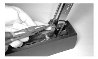
**58. Slip the chrome cover over the shift lever**, but temporarily support it as far upward and rearward as possible. Then reinstall the trigger assembly, the brass washer, and the spring clip.
