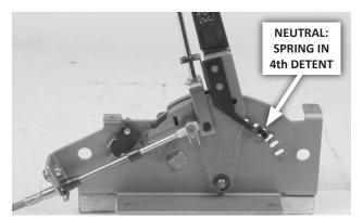
A. With the selector lever still in NEUTRAL (2 clicks from PARK) and the shifter in the NEUTRAL position (shown), adjust the cable bracket nuts (and swivel, if necessary) until the swivel slips freely in and out of the selector lever hole.
