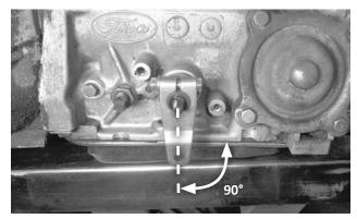
28. Install the B&M selector lever using the 1/4-20 × 1-1/2" bolt, lock washer and nut. (See NOTE on next page.) With the selector shaft still in NEUTRAL, align the selector lever perpendicular to the oil pan split-line, then tighten the fasteners.
