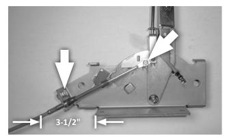
Assemble the cable and shifter. Secure the cable eye to the shifter pin with the 3/32" (large diameter) cotter pin. Then secure the cable's mount tab to the outside surface of the shifter base with the 1/4-20 × 1/2" bolt and nut (apply medium strength thread-locking fluid to the bolt).
