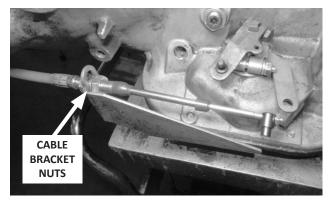
**15.** Attach the shifter cable to the cable bracket: First remove the small jam nut, both plastic dust boots, and one large nut and lock washer, from the cable. Then insert the cable through the cable bracket, reinstall the lock washer and nut (loosely, to allow room for adjustment), and reinstall the dust boots.
