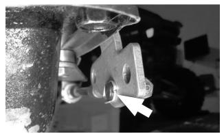
**48.** Secure the swivel to the selector lever with the **1/16**" (small-diameter) cotter pin. Operate the shifter through all the gear positions, verifying that it operates correctly.
