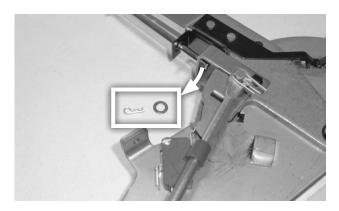
54. Remove the T-handle and jam nut from the shifter, then remove the lockout trigger by removing both the spring clip and the brass washer from the bottom end of the rod.
