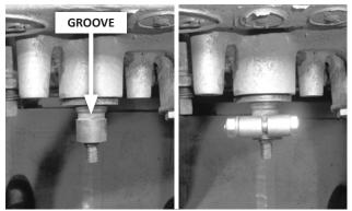
**NOTE:** If the selector shaft is grooved as shown, center the lever between the groove and the end of the shaft, so that the lever's inboard clamping surface does not land in the groove.
