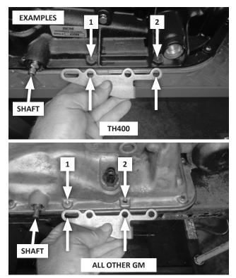
**42.** Check cable bracket fit: Remove the two oil pan bolts to the rear of the selector shaft. Determine which cable bracket holes will be used on your transmission.
