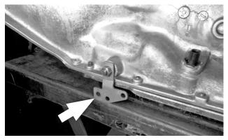
**41.** Install the B&M selector lever using the stock selector lever nut, and tighten the nut to 23 ft-lbs torque. The lever should travel smoothly back and forth, with a positive "click" in each detent.
