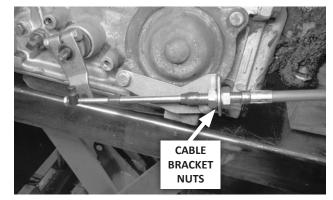
**30.** Attach the shifter cable to the cable bracket: First remove the small jam nut, both plastic dust boots, and one large nut and lock washer, from the cable. Then insert the cable through the cable bracket, reinstall the lock washer and nut (loosely, to allow room for adjustment), and reinstall the dust boots.
