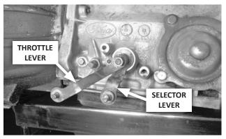
**25.** Disconnect stock controls: Remove and retain the nut and lock washer holding the throttle lever on its shaft. Carefully remove the throttle lever, and move it and its linkage aside, allowing them to hang free. Remove and discard the stock shift linkage.
