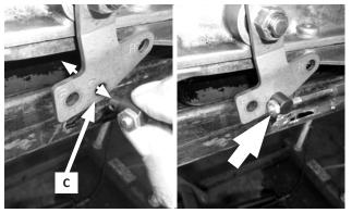
B. Gradually tighten the cable nuts against the bracket while continuing to check the fit of the swivel in hole "C" in the selector lever. Then with the swivel inserted in the selector lever, lightly snug the jam nut.
