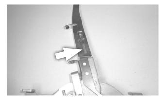
**57. Install the red position indicator tape** on the left side of the shift lever, as shown — just below the rear leg of the letter "M," and parallel to the rear edge of the lever.
