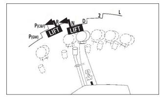
The lockout trigger must be lifted to move:
