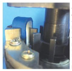
ECU. Make sure the rotor is in the center position and that it is pointed at the mark you made for the #1 spark plug location. Remove the rotor if it helps you see the reluctor position better.
