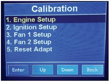
The Calibration screen will appear. On the Calibration screen, select #1 Engine Setup.
