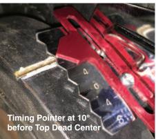
evant for this setup example. Drop your distributor in place like you normally would with the rotor pointing at the #1 spark plugposition.
