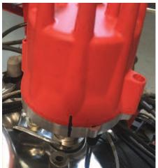
4- Line up the center of the reluctor wheel (this is the 8 paddle wheel) with the center of the pickup on the distributor. See the photo at bottom of page. Use a light to make sure you are centered and snug down the
